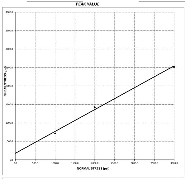
Shear Strength:  $\Phi = 31^{\circ} C = 175 \text{ psf}$
