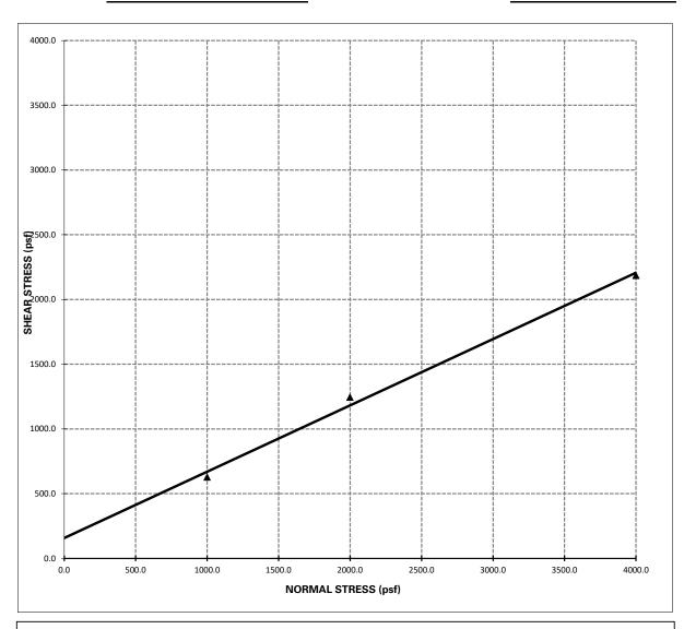
Shear Strength:  $\Phi = 27^{\circ}$ , C = 158 psf
